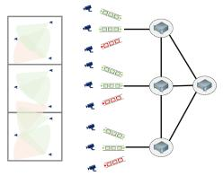
Figure 1: Typical scenario where cameras in each area are associated to an entry point.
